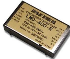
LMD-400-R is a synthesized transceiver with 10 mW RF power, 4800 bps data rate and GFSK modulation. It is designed for use in the license bands in Europe and the U.S.A. that require the high receiver performance and narrow band transmission shown below.
